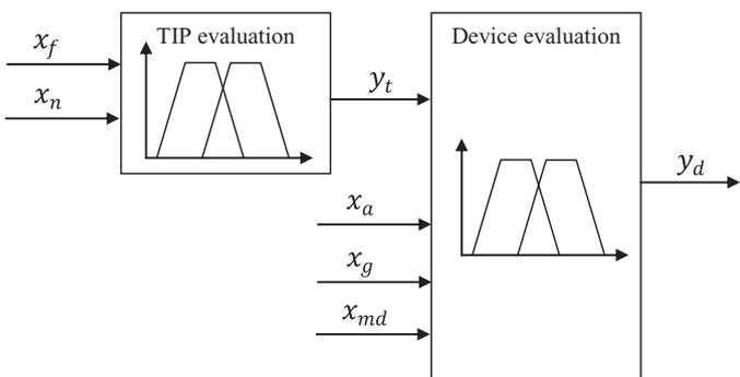
Fig. 3. Diagram of the Device evaluation fuzzy model.
