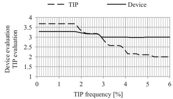
**Fig. 12.** Relation between the *TIP Evaluation* and *Device Evaluation* variables and the *TIP Frequency* variable for the Heimann Smiths 6046 si device.
