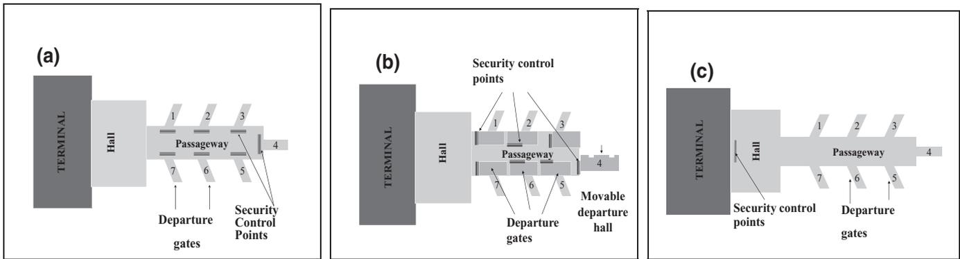
Fig. 1. Security control structures (a - at the departure gate, b - decentralised system, c - centralised system).
