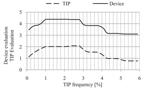
**Fig. 11.** Relation between the *TIP Evaluation* and *Device Evaluation* variables and the *TIP Frequency* variable for the Smiths Detection 10080 EDX-2is.
