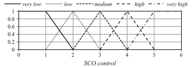
Fig. 6. Linguistic membership functions of the output variable SCO control.
