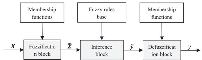
Fig. 3. General structure of the fuzzy inference system.
