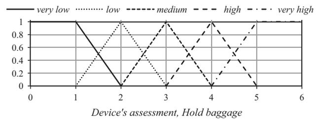
**Fig. 7.** Membership functions of the linguistic variables *Device's assessment* and *Hold baggage*.
