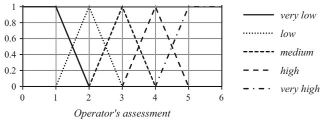
Fig. 4. Linguistic membership functions of the output variable *Operator's assessment*.
