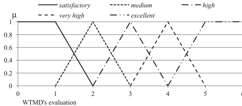
Fig. 3. Membership functions of the WTMD's evaluation output variable.
