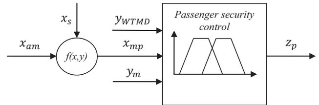
Fig. 2. Structure of the Passenger security control fuzzy model.
