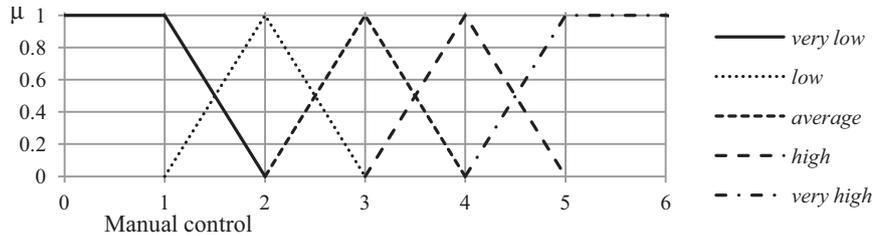
Fig. 8. Membership functions of the *Manual control* model output variable.
