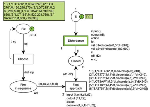
Figure 1. CSPN model for scheduling assessment—aircraft input and disturbance appearance.
